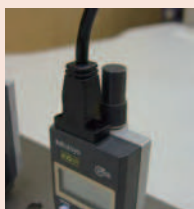
ABS Digimatic Indicator ID-N with 02AZD790G cable
