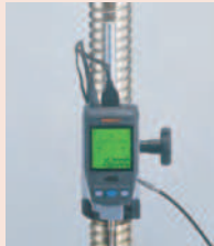
Digimatic Indicator ID-H with 02AZD790D cable
