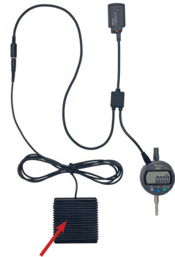
Cable with footswitch connection
