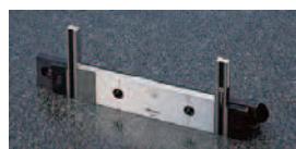
Holder B and C : Used for coupling two long gauge blocks together with other gauge blocks up to 35 mm (Holder B) or 140 mm (Holder C). Also used for attaching jaws with two adapters.
