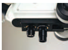
Using optional slide type nosepiece with 2-lens mount (factory-fit option)
