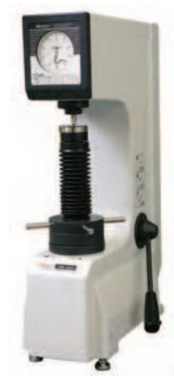
HR-110MR Rockwell hardness testing machine An environmentally friendly energy-saving model. The basic operation is all manual, including weight-changing (total test force selection).
