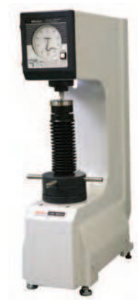
HR-210MR Rockwell hardness testing machine Manual weight changing (with total test force selected) and handling of preload force. Motor drive controls loading sequence.
