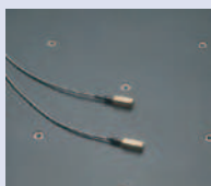
Temperature compensation system (photo : temperature sensors)
