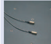
Temperature compensation system (photo : temperature sensors)
