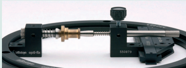
Holding a cylindrical part between clamping tips.
