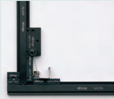
Toothed rule that lets light pass Spring flange locking the part in the measurement position.
