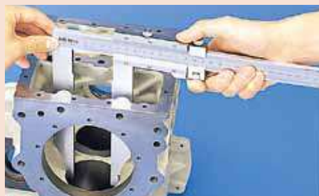
Radiused jaws for accurate ID measurement
