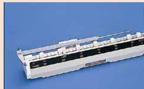
Checking the accuracy of a caliper
