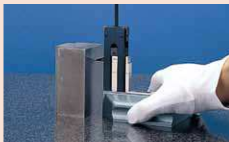
Marking a workpiece using the base, a holder and the scriber point.
