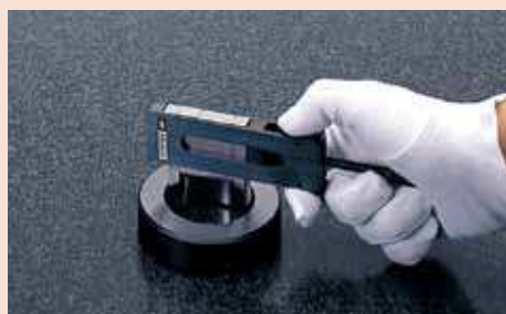
Gauging a bore using a pair of half round jaws and a holder.
