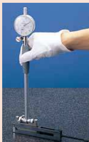
Setting a bore gauge using a holder with the pair of Type I half-round jaws arranged as flat contact surfaces.
