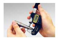
Thanks to the quick movement, positioning times are reduced by 60%\* and measuring times by 35%\* compared with a conventional micrometer.
