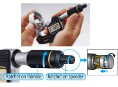
Ratchet-induced micro-vibrations along the spindle help ensure repeatable measurements.
