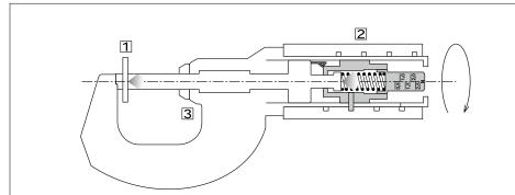
D Measuring force is generated by the action of trapping a workpiece between the spindle face and the anvil. 2 The constant-force unit applies the specified measuring force.
