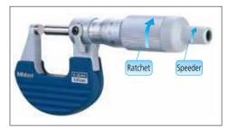
• Rotating the thimble/speeder when the workpiece is between the anvil and spindle causes the ratchet mechanism to operate and apply a constant measuring force to the workpiece.
