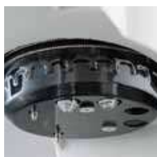
Power turret with 2 indenter mounts and 4 objective mounts (manual operation possible)
